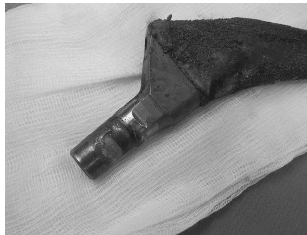
Fig. 3 Severe corrosion of the taper in a Taperloc® stem (Biomet) is shown.
