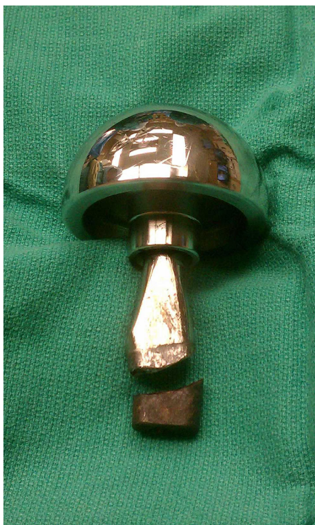
Fig. 2 A corroded, long varus modular neck with fracture is shown. The broken fragment was removed from the stem to allow attachment of an extraction device to remove the stem.
