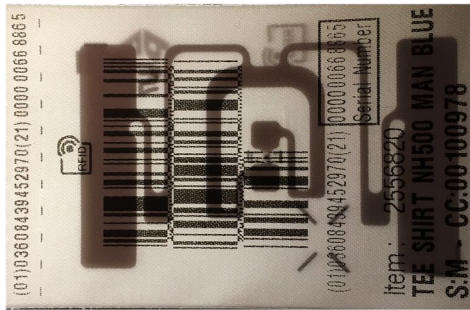
Fig. 1 Clothing label with a passive RFID tag shining through (© Ulrike Felt) and icon informing consumers that RFID tags are in use ( https://www.aim-d.de/wp-content/uploads/Emblem_rfid-generic.jpg )
