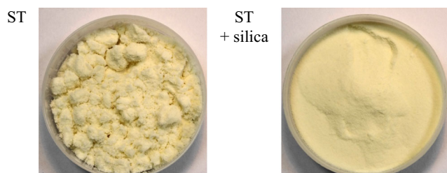
Fig. 2 Images of microencapsulated oil ST powder with and without addition of silica Aerosil
