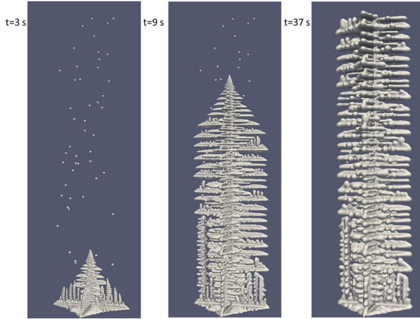
Fig. 1. Growth of an alloy 718 dendrite at a primary spacing \lambda_1 = 250 \mu\text{m} .
