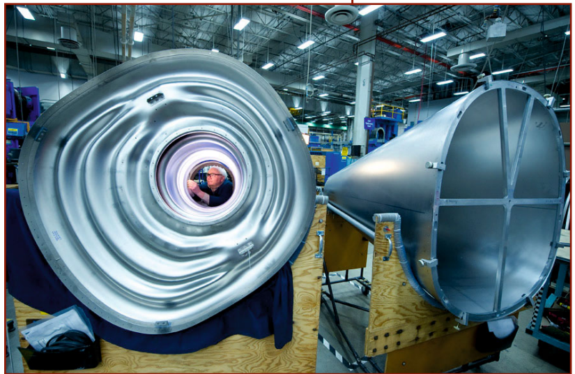
Dan Sanders at work at Boeing, examining a titanium tail cone assembly for the 787 Dreamliner. (Photo: Robert Ferguson, Boeing)
