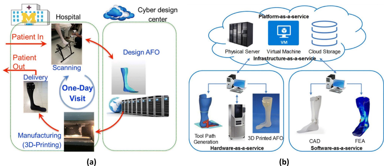
Fig. 30 a Overview of the Cyber Design and Additive Manufacturing (CDAM) system for custom Ankle Foot Orthoses (AFO). b Illustration of the interaction between the hardware and software systems with the cloud storage system [297]
