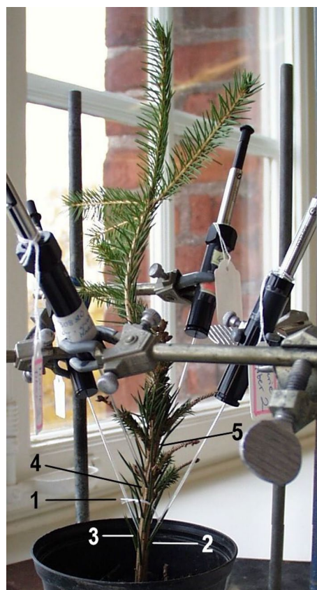
Fig. 1 Single needle collection setup. (1) MeJA solution was applied at the lowest 5 cm of the stem. (2, 3) Needles growing on the MeJA-treated area, covered with thin glass tubes with SPME's holders mounted and fibres exposed inside. (4) needle growing 1 cm above the treated area. (5) Needle growing 2 cm above the treated area. SPME holder and glass tube mounted against the stem 10 cm above treated area
