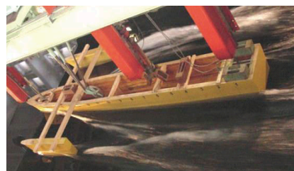
Figure 10 Picture of Kelvin's wave systems in the experiment
