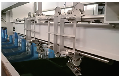
Figure 12 Four-component measuring instrument
