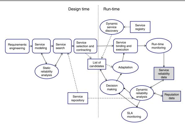
Fig. 1 Reliable composite service design and run-time modeling
