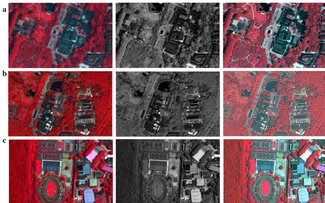
Fig. 3 Image fusion results. a QuickBird image; b IKONOS image; c WorldView2 image. Left: multispectral image; middle: panchromatic image; right: fused image ( a HSV; b wavelet transform with wavelet basis of bior2.8; c wavelet transform with wavelet basis of coif1)
