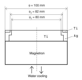
Fig. 1 Schematic of composed Ti/Ag magnetron target
