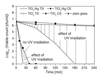
Fig. 10 Colony forming units (cfu/ml) on surface of plain glass, glass coated with TiO<sub>2</sub> (commercial TiO<sub>2</sub>) with (TiO<sub>2</sub> TS) and without (TiO<sub>2</sub> CS) UV irradiation, and TiO<sub>2</sub>/Ag single layer with (TiO<sub>2</sub>/Ag TS) and without (TiO<sub>2</sub>/Ag CS) UV irradiation as a function of irradiation time
