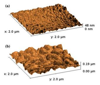
**Fig. 6** Comparison of AFM surface topography of **a** thin (~700 nm) and **b** thick (~1,500 nm) Ti–Ag–O films sputter-deposited on unheated glass substrate at  $I_{\rm D} = 2$  A,  $U_{\rm S} = U_{\rm fl}$ ,  $d_{\rm s-t} = 120$  mm,  $p_{\rm T} = 1.5$  Pa and  $p_{\rm O_2} = 0.9$  Pa
