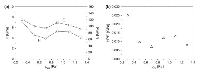
Fig. 9 a Microhardness H and effective Young's modulus  $E^*$  and b ratio  $H^3/E^2$  of ~950 nm thick Ti-Ag-O films as a function of partial pressure of oxygen  $p_{O_2}$ . Deposition conditions:  $I_D = 2$  A,  $U_S = U_{\text{fl}}$ ,  $d_{s-t} = 120$  mm
