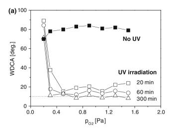
Fig. 7 Characterization of water droplet contact angle WDCA on the surface of **a** thin ( $\sim$ 700 nm) and **b** thick ( $\sim$ 1,500 nm) Ti–Ag–O films under UV irradiation for 20, 60 and 300 min as a function of
