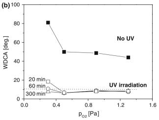
partial pressure of oxygen  $p_{O_2}$ . Deposition conditions:  $I_D = 2$  A,  $U_S = U_{\rm fl}, d_{\rm s-t} = 120$  mm, unheated glass substrate
