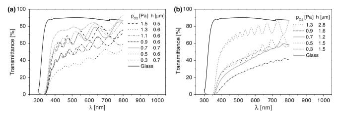
Fig. 8 Transmission spectra of **a** thin (~700 nm) and **b** thick (~1,500 nm) Ti–Ag–O films sputter-deposited on unheated substrates as a function of  $p_{O_2}$ . Deposition conditions:  $I_D = 2 \text{ A}$ ,  $U_S = U_{fl}$ ,  $d_{s-t} = 120 \text{ mm}$
