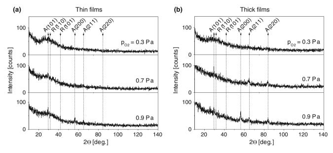
Fig. 5 Comparison of X-ray structure of **a** thin (~700 nm) and **b** thick (~1,500 nm) Ti-Ag-O films sputter-deposited on unheated glass substrate at  $I_D = 2$  A,  $U_S = U_{fl}$ ,  $d_{s-t} = 120$  mm,  $p_T = 1.5$  Pa and three values of  $p_{O_2} = 0.3$ , 0.7 and 0.9 Pa
