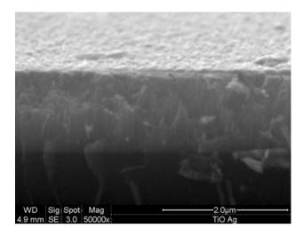
**Fig. 4** Cross-section SEM image of thick (~1,500 nm) Ti-Ag-O film sputter-deposited on unheated substrate at  $I_{\rm D} = 2$  A,  $U_{\rm S} = U_{\rm fl}$ ,  $d_{\rm s-t} = 120$  mm,  $p_{\rm T} = 1.5$  Pa and  $p_{\rm O_2} = 0.5$  Pa
