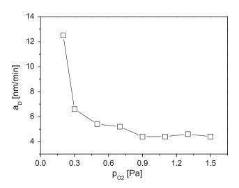
**Fig. 2** Deposition rate  $a_{\rm D}$  of reactively sputter-deposited Ti–Ag–O films as a function of  $p_{\rm O_2}$ . Deposition conditions:  $I_{\rm D} = 2$  A,  $U_{\rm S} = U_{\rm fl}$ ,  $d_{\rm s-t} = 120$  mm,  $p_{\rm T} = 1.5$  Pa
