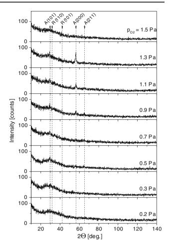
**Fig. 3** XRD patterns from ~500 to 700 nm thick Ti–Ag–O films sputter-deposited at  $I_{\rm D} = 2$  A,  $U_{\rm S} = U_{\rm fl}$ ,  $d_{\rm s-t} = 120$  mm on unheated glass substrate, as a function of  $p_{O_2}$
