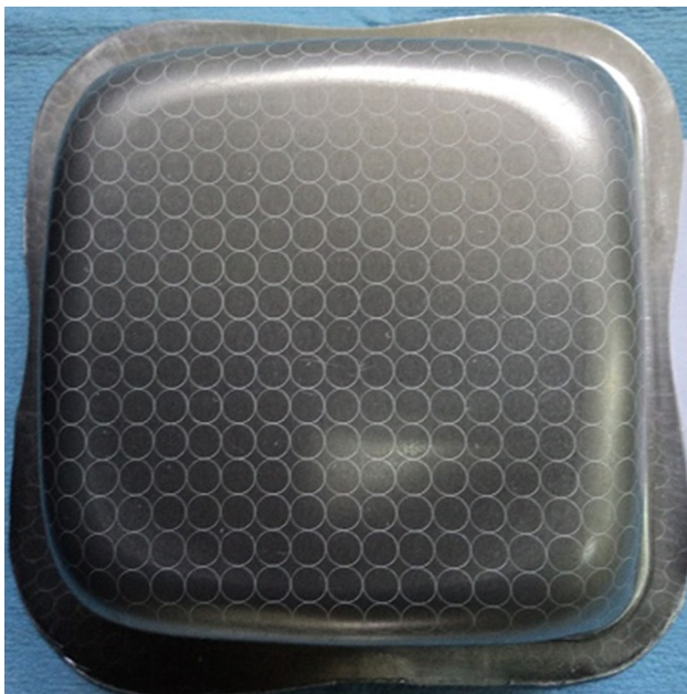
Fig. 9 Square cup hydroformed with 23.5 MPa peak pressure and 10 kN BHF
