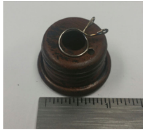
Fig. 2 Tabletop torch cap showing the 2 mm vent hole and torsional spring clip that is used to hold the wick
