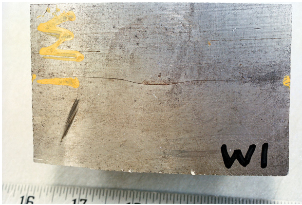
Fig. 13 Piece of roll, as removed at location of crack in roll at balance weight screw location
