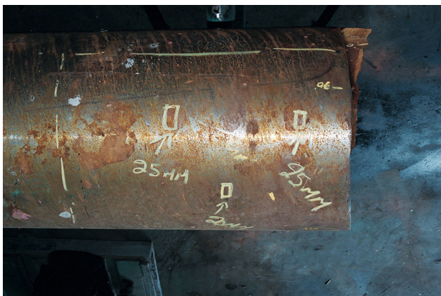
Fig. 3 Fractured end of roll, located 70 in (1778 mm) from one end
