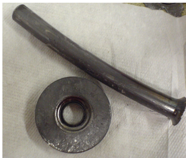
Fig. 3 Extrusion die and a rod after hot direct extrusion
