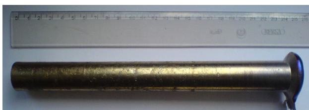
Fig. 1 The 900 g NiTi ingot obtained after vacuum induction melting
