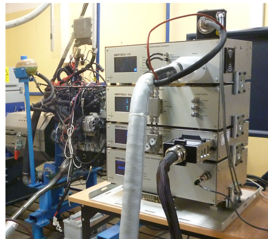
Fig. 2. SEMTECH ECOSTAR instrument, used to measure emissions in accordance with the RDE methodology.
