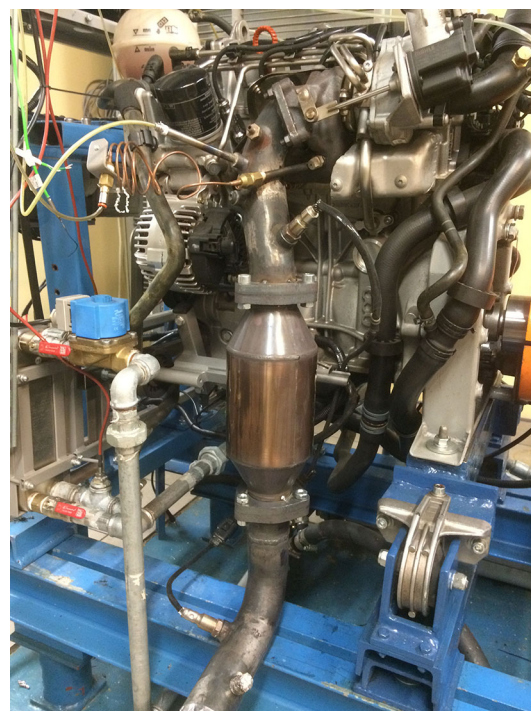
Fig. 1. 1.2-dm 3 TSI combustion engine chosen for this research.
