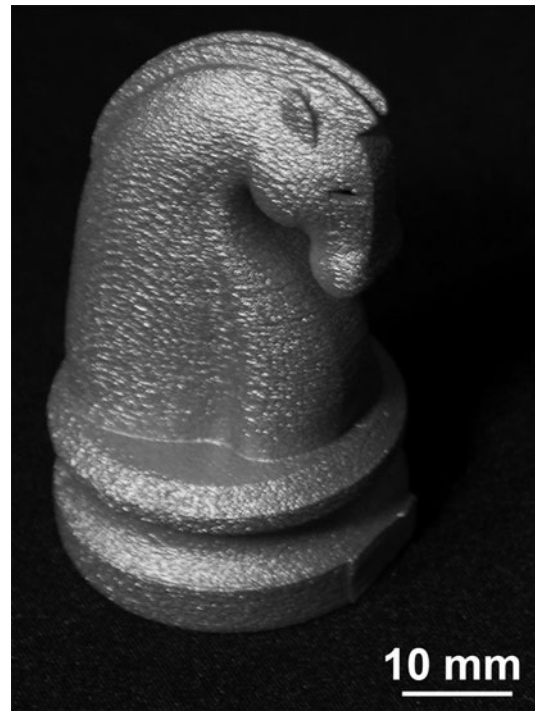
Fig. 9—A closed-pore aluminum part made by selective laser sintering, nitridation at 833 K (560 °C), and an open-closed pore transformation treatment at 973 K (700 °C).
