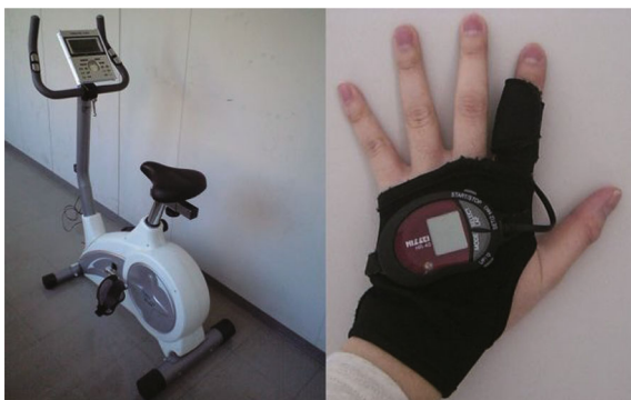
Fig. 2 Left: programmable ergometer, AFB6008; Right: photoelectric heart rate meter, Pulse Coach Neo HR-40
