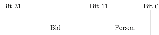
Fig. 4 Example of a partitioning of a value stored in the bidding array. In this case, a 32-bit data type is assumed. The 20 highest bits are used to store the current bid and the 12 lowest for the person
