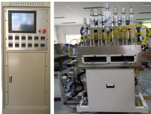
Fig. 20 Photograph of glass molding machine PFLF7-60A (SYS Co., Ltd., Japan)
