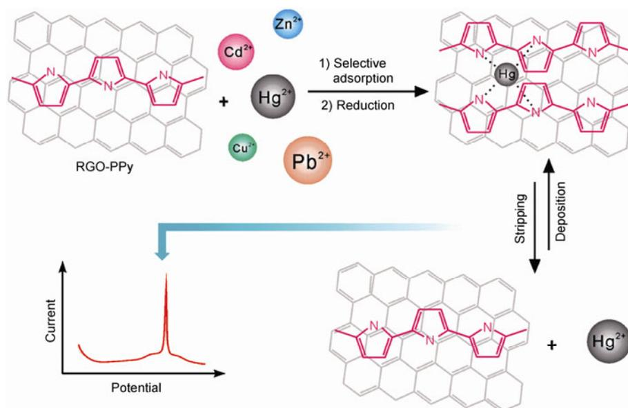
**Figure 7** (Color online) A schematic drawing of  $\text{Hg}^{2+}$  electrochemically selective detection by the PPy-RGO nanocomposite. Reprinted from ref. [85] with permission from the Royal Society of Chemistry.
