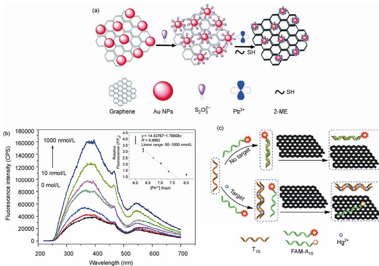
**Figure 5** (Color online) (a) The sensing mechanism for  $\text{Pb}^{2+}$  and (b) the fluorescence spectra of  $\text{Pb}^{2+}$  ( $0$ – $1.0 \times 10^{-6}$  mol  $\text{L}^{-1}$ ) of G-AuNCs. Reprinted from ref. [76] with permission from the American Chemical Society. (c) The schematic illustrating the fluorescence detection of  $\text{Hg}^{2+}$  based on DNA duplexes of poly(dT) and GO. Reprinted from ref. [82] with permission from Royal Society of Chemistry.
