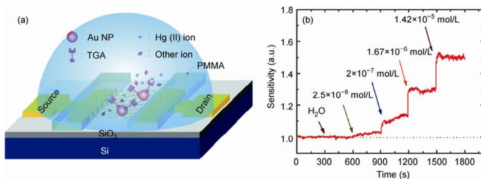
**Figure 6** (Color online) (a) The schematic diagram and (b) the dynamic response for  $\text{Hg}^{2+}$  of the rGO/TGA-AuNP hybrid sensor. Reprinted from ref. [84] with permission from the American Chemical Society.
