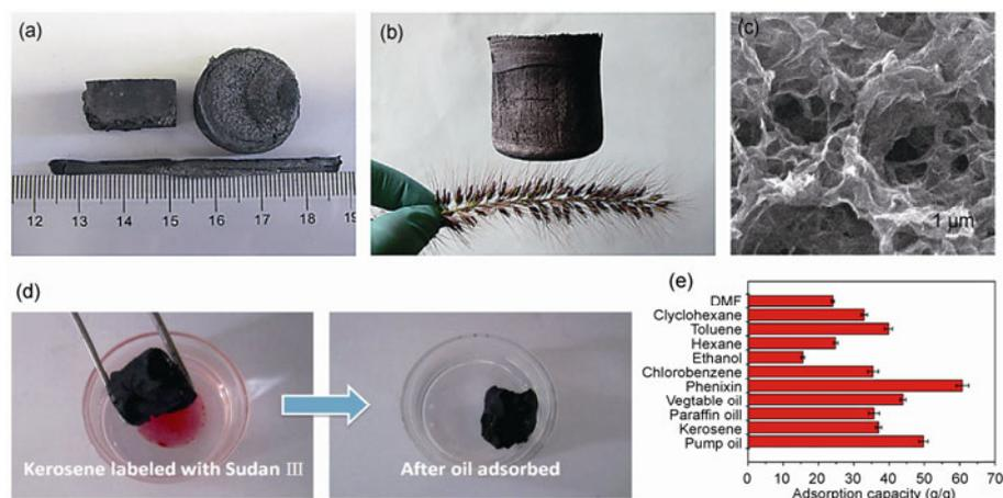
**Figure 3** (Color online) (a), (b) Macroscopic structures of ultra-flyweight aerogels with diverse shapes. Reprinted from ref. [34] with permission from the WILEY-VCH Verlag GmbH & Co. kGaA, Weinheim; (c) SEM image; (d) photograph of the kerosene labeled with Sudan III adsorption; (e) adsorption capacities for different oils and organic solvents at saturated state of GaA-GA. Reprinted from ref. [35] with permission from the Royal Society of Chemistry.
