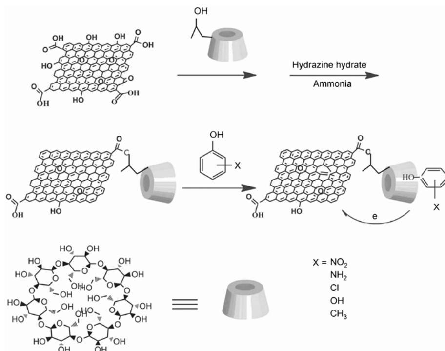
**Figure 8** Schematic of the synthesis process of HP-β-CD-RGO composites and the interaction between the guest (*o*-nitrophenol) and the host (cyclodextrin moiety linked up to RGO). Reprinted from ref. [91] with permission from the Royal Society of Chemistry.
