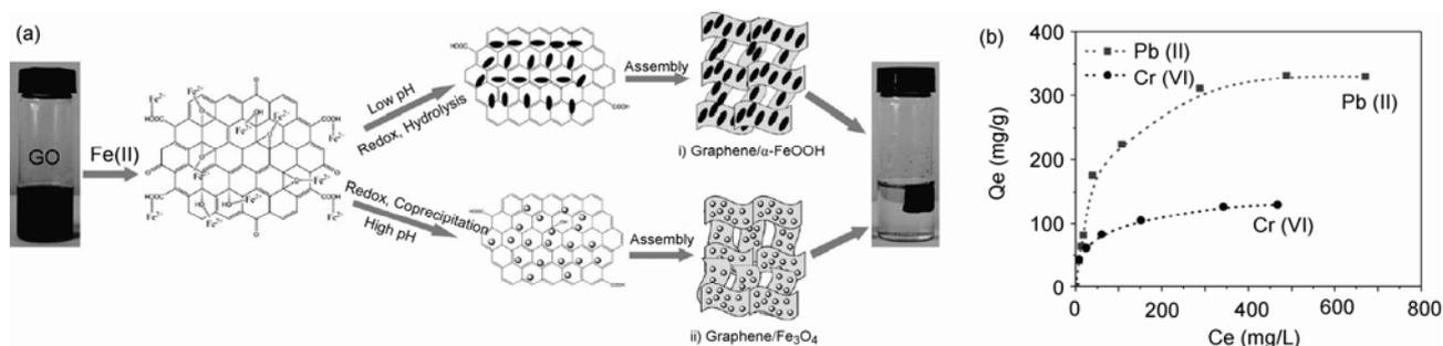
**Figure 2** (a) The formation mechanism of graphene/iron oxide hydrogel; (b) the adsorption isotherms of  $\text{Cr}^{6+}$  and  $\text{Pb}^{2+}$  on graphene/FeOOH hydrogel at room temperature. Reprinted from ref. [27] with permission from the American chemical Society.
