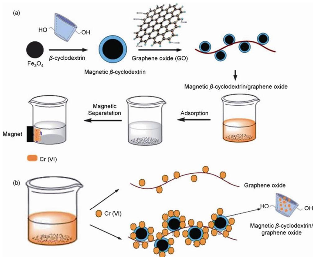
**Figure 1** (Color online) (a) The synthesis and application for removing  $\text{Cr}^{6+}$  of MCGNs. (b) the comparison of adsorption mechanisms on GO and MCGN. Reprinted from ref. [25] with permission from the Royal Society of Chemistry.
