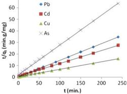
Fig. 26 Pseudo-second-order kinetic model for biosorption of lead, cadmium, copper, and arsenic onto algal biomass
