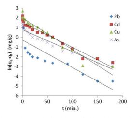
Fig. 25 Pseudo-first-order kinetic model for biosorption of lead, cadmium, copper, and arsenic onto algal biomass
