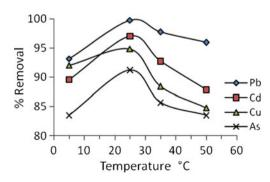
Fig. 7 Variation of percentage removal with temperature, pH=4,  $C_i$ = 50 mg/l for each metal
