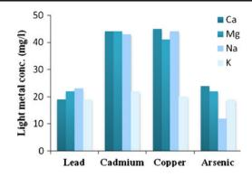
Fig. 2 Amounts of light metals released due to heavy metal biosorption,  $C_i=50$  ppm, contact time 4 h at 200 rpm
