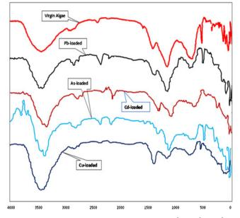
Fig. 1 FTIR spectra obtained for virgin algae and Pb<sup>2+</sup>-, Cd<sup>2+</sup>-, Cu<sup>2+</sup>-, and As<sup>3+</sup>-loaded algae
