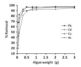
Fig. 5 Biosorption efficiency at optimum pH value for  $Pb^{2+},\,Cd^{2+},\,Cu^{2+},\,and\,As^{3+}$
