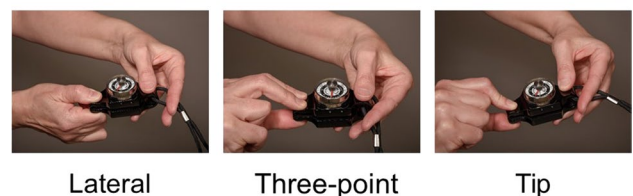
Fig. 2 Pinch test. In the pinch test, the patient pinches the measurement device in three different positions as tightly as possible
