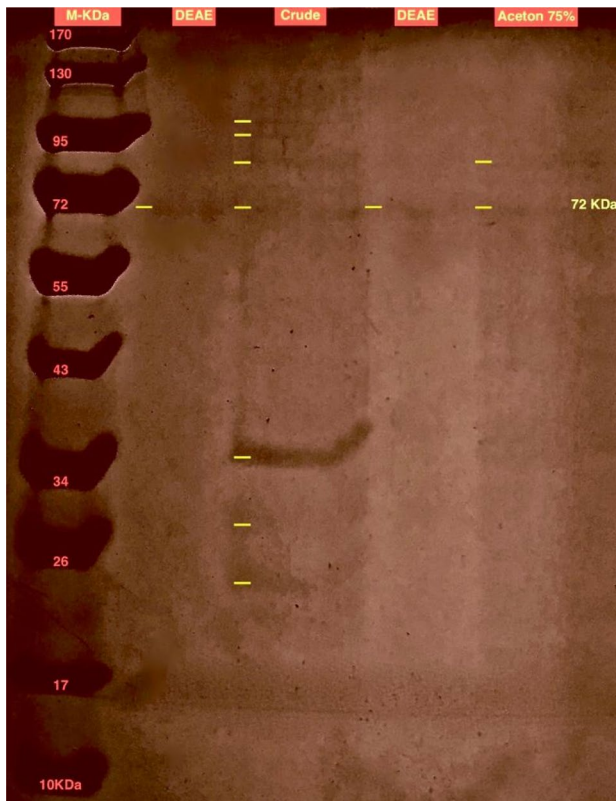
Fig. 2 SDS-PAGE of samples during purification of \beta -1,3-1,4-glucanase from Halomonas meridiana ES021. The standard protein marker (Page Ruler prestained protein ladder (10–170 kDa)). Lane 1&3: replica for the fraction eluted from DEAE-Cellulose A-52 column (pure enzyme); lane 2: culture supernatant (crude enzyme); lane 4: 75% acetone fraction (semi-purified enzyme)
