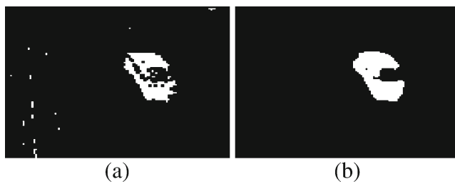
Figure 4 An example of the operation of the Hough transform block: a —image m_{BEHSX} before Hough block, b —image m_V after Hough block.
