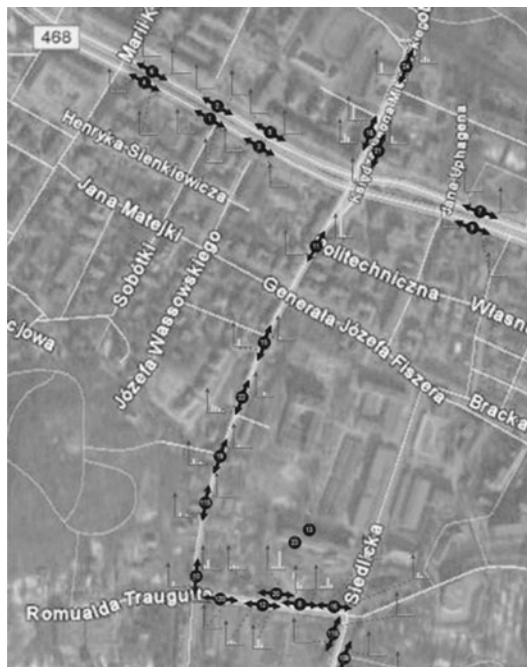
Figure 21 The location of the sensor network nodes (black dots) on the streets. The arrows indicate the directions of measured traffic.
