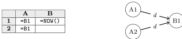
Fig. 5 Two cells depend on the same cell containing a call to NOW() . If both cell A1 and A2 are evaluated in parallel and both recursively attempt to evaluate B1, their respective threads must agree upon which value B1 has evaluated to
