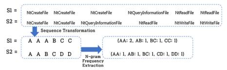
Fig. 3 n-gram-based comparison set extraction
