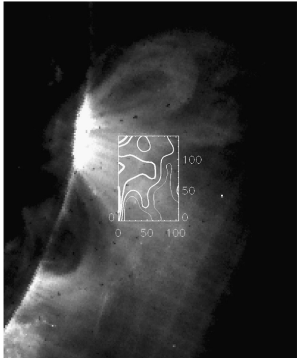
Fig. 1 Contour map of the measured coronal magnetic field strength using Fe XIII overplotted on the EIT Fe XV image. The thick contour corresponds to 4 G, with additional contours corresponding to flux densities of 2, 0, and -2 G. Here the line-of-sight magnetic flux density and transverse field orientation were mapped in two dimensions with a sensitivity of about 1 G and 20'' spatial resolution after 70 minutes of integration. These measurements reveal the line-of-sight coronal magnetic field 100 Mm above an active region to have a flux density of about 4 G. From Lin et al. (2004), Fig. 3. © AAS. Reproduced with permission
