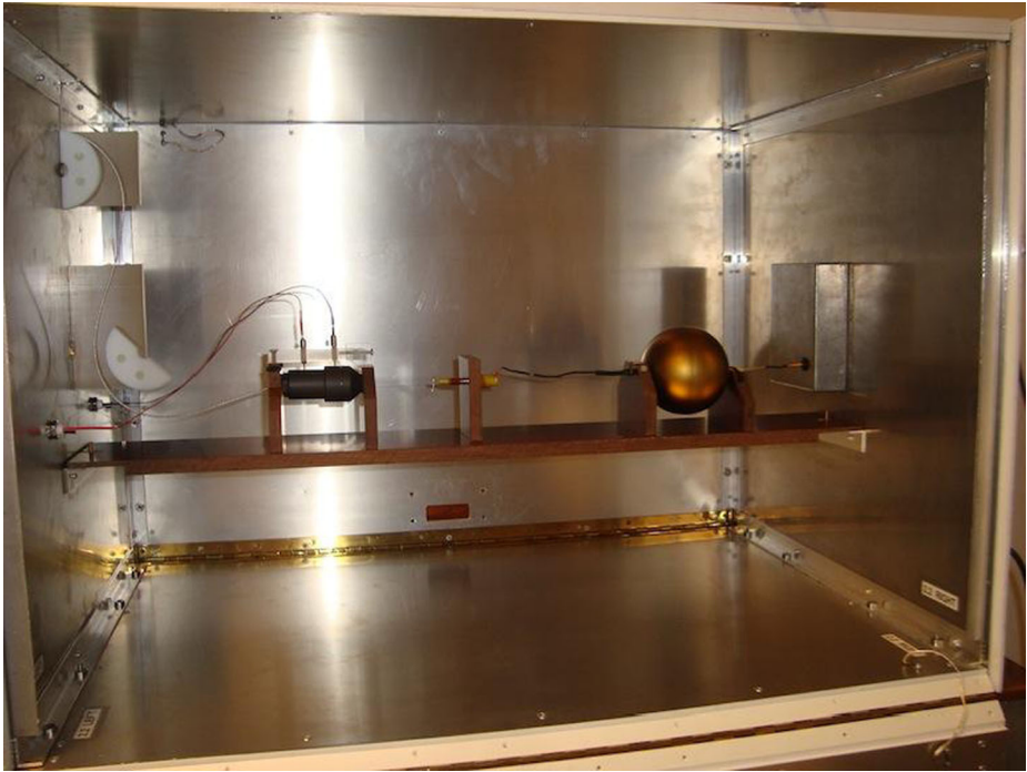
Fig. 27 The FM2 preamp mounted in the test stimuli box at IRFU for thermal verification testing, stage 1
