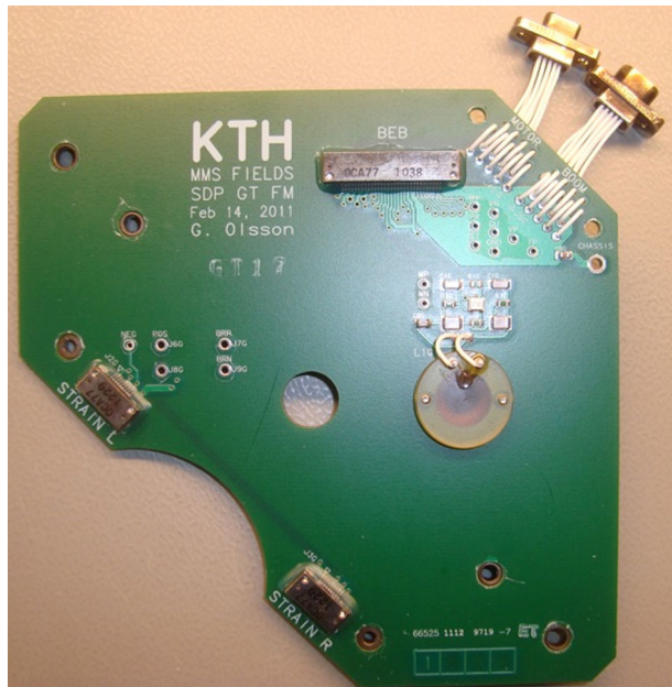
Fig. 16 Photo of FM17 BEB GT board with inductive sensor
