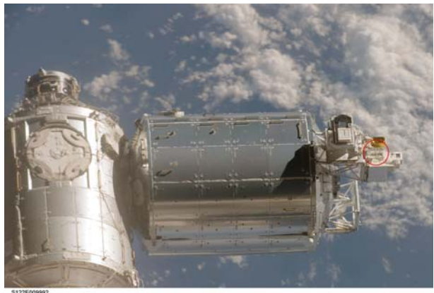
Fig. 5 EXPOSE-E after being installed on the EuTEF platform at the balcony of the European Columbus module of the ISS in February 2008, before commissioning and opening of the lids (credit ESA and NASA), see also ( http://www.go.dlr.de/musc/expose/ )
