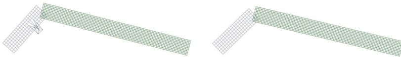
Fig. 3 Mesh distortion due to flying elements ( left ). No flying elements due to scaling the element mass ( right )
