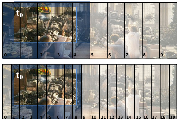
Fig. 2 Finer ( bottom ) and coarser ( top ) tiling and impact on pixel overhead
