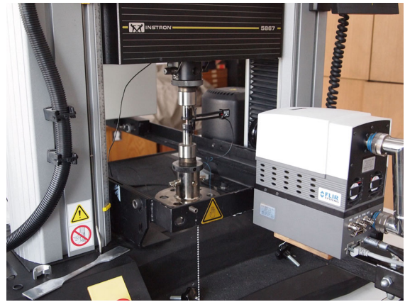
Fig. 1 Photograph of the experimental set up: FSMA single crystal sample in grips of Instron testing machine and FLIR System infrared camera
