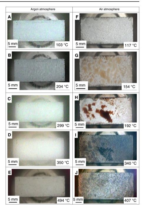
comparison to those sintered under the argon atmosphere. Above a temperature of 400 °C no sample changes were observed, although on the sample's surface many small black discolorations as the effect of material oxidation, were determined.
