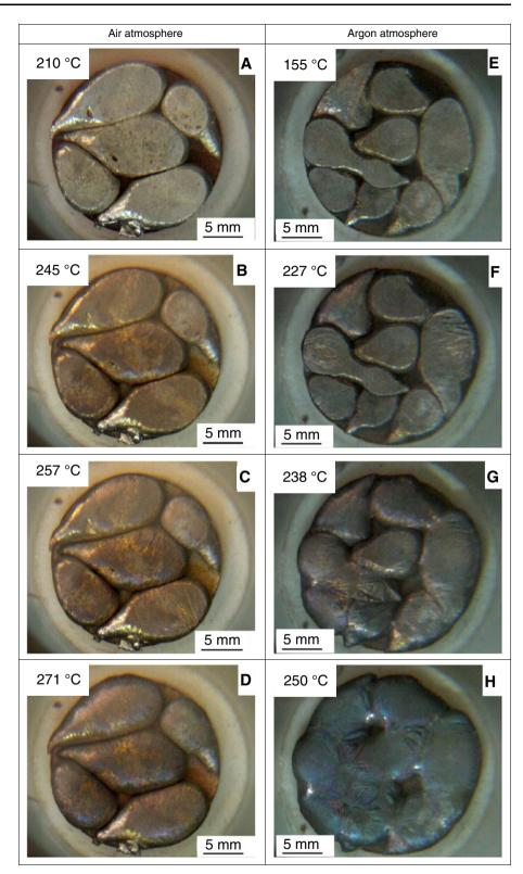
oxidation, changed their shape at 227 °C (spheroidization, Fig. 6f) and at 238 °C (Fig. 6g) the local merging point started taking place. A further temperature rise resulted in growth of the existing connections and the creation of new necks in studied material. In general, this effect can be
