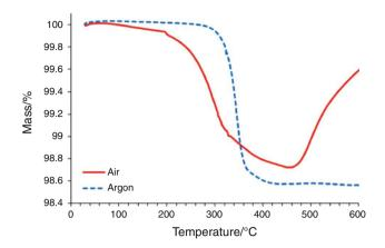
Fig. 4 TG curves for the Alumix 431D powder heated in argon and air atmosphere
