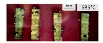
Fig. 5 Spherical bubbles on the sample surface as an effect of partial material oxidation during the heating process
