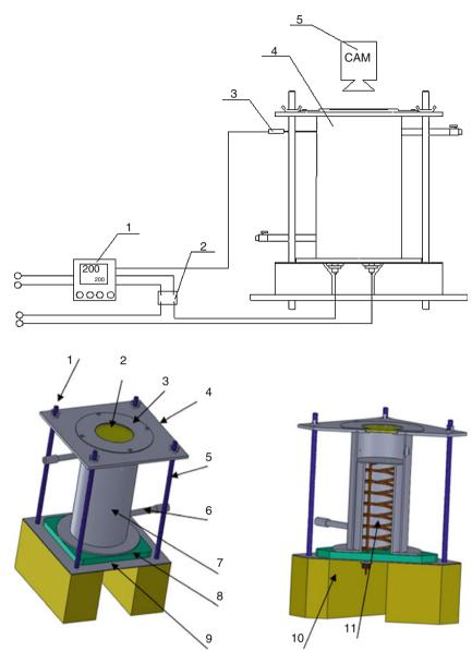
**Fig. 2** 3D visualization of the body of the device: *1* pressure bolts, *2* observing glass, *3* pressure ring, *4* top plate, *5* threaded rods, *6* channel inlet gas, *7* housing, *8* insulating pad, *9* base plate, *10* support, *11* heater
