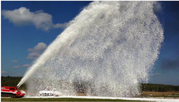
Fig. 8 FHF delivery by fire-fighting tracked vehicle “Yamal-201” (reprinted with permission from Vinogradov AV, Kuprin DS, Abduragimov IM, Kuprin GN, Serebriyakov E, Vinogradov VV (2015) Silica foams for fire prevention and firefighting. ACS Appl Mater Interfaces 22 October 2015. Copyright 2015 American Chemical Society)
