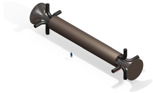
Fig. 1 A 3D view of the theoretical device studied in this paper, with fission mantle, coolant outflow pipes and magnetic expanders at the ends
