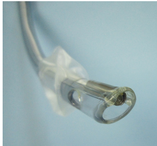
Fig. 2 A camera and a light source embedded at the tip of EtView tracheal ventilation tube
