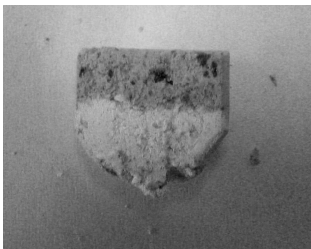
Fig. 9 Cross-section of powder distribution following extrusion of paste with initial LPR = 0.425 through tapered barrel exit, \theta_{\text{exit}} = 45^\circ , at a plunger rate of 10 mm/min
