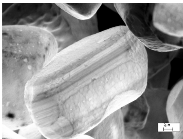
Fig. 3 CL image of ACCEL phosphor particles
