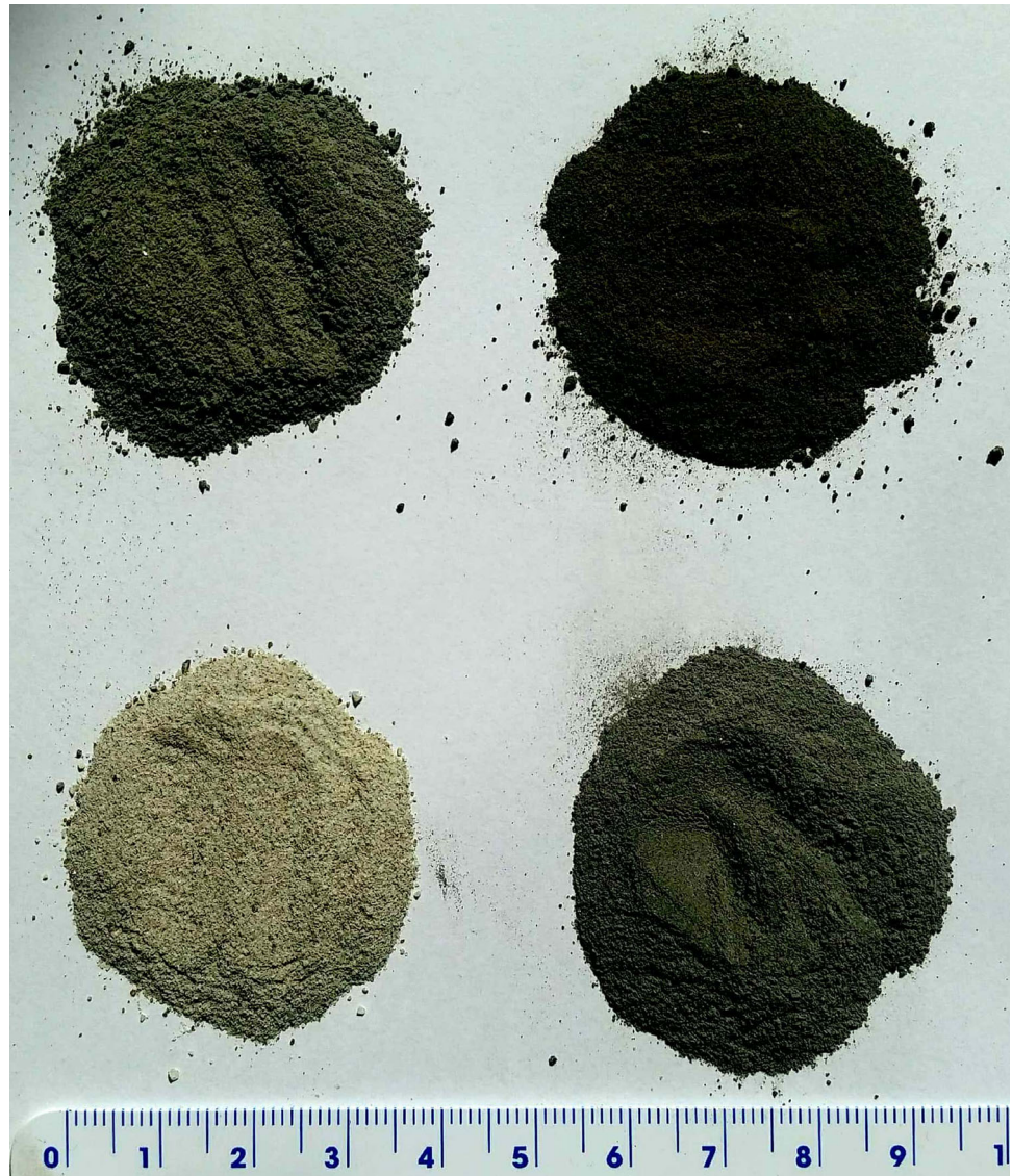
Figure 1 Four types of lunar regolith used: EAC-1 (top left), JSC-2A (top right), LHT-3M (bottom left), FJS-1 (bottom right). Scale bar is in cm.
