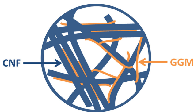
Fig. 5 Schematic illustration of nanofibrillar network in CNF/GGM nanocomposite. Note that the solid materials will have very low porosity
