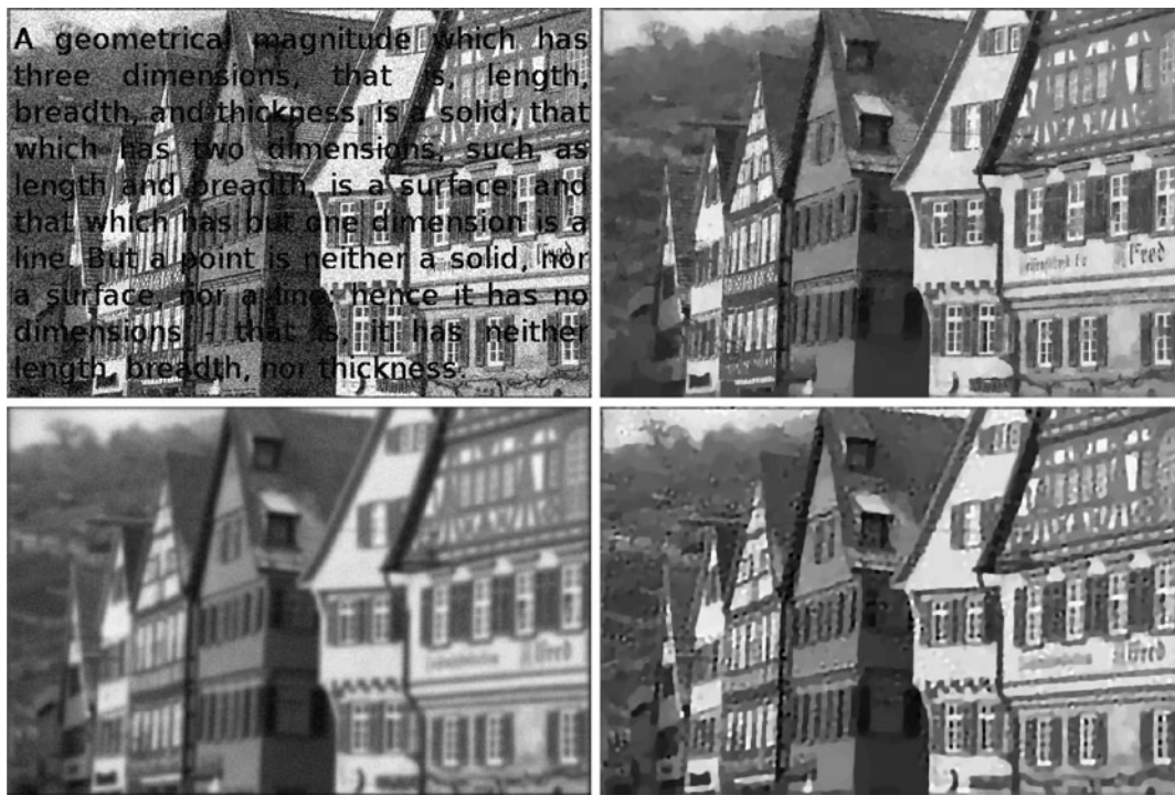
Fig. 9 Inpainting (top): data Y with \sigma = 0.1 (left) and SMRE (right). Deconvolution (bottom): data Y with \sigma = 0.02 (left) and SMRE (right)
