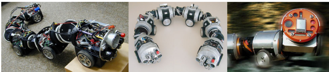
Fig. 4 MAKRO robots for sewer inspection (from left): MAKRO 1.0, MAKRO 1.1, MAKROplus (reproduced from [15, 51])
