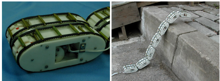
Fig. 8 Prototype of Millibot Train: detail of a single module 3 cm high \times 5 cm wide \times 10 cm long (left), seven modules climbing a double-height (33 cm) step (right), The Robotics Institute, Carnegie Melon University
