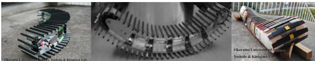
Fig. 17 Flexible mono-tread mobile robot RT02-WORMY (from left): laterally flexed, retroflexed, twisted (Yoshida & Kinugasa Lab, Okayama University of Science)
