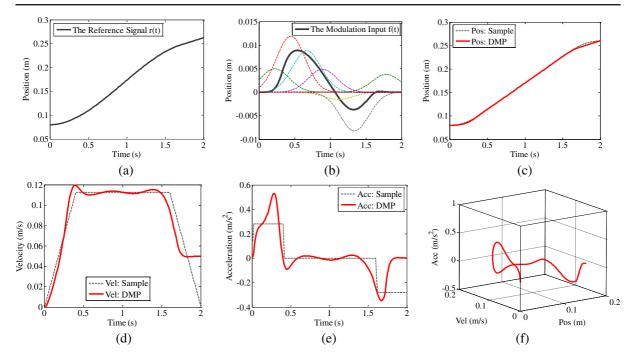
**Fig. 6** 1-DOF case. **a** Reference signal r(t). **b** Gaussian Kernels and the final modulation signal f(t). **c**-**e** Generated trajectory result and the provided sample trajectory
