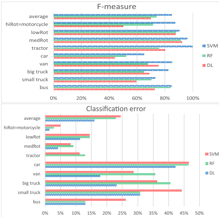
Fig. 7 F-measure and classification error for each binary classifier in hierarchical classification, using features above the threshold in feature selection
