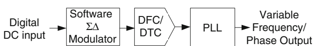
Fig. 2 Phase/frequency test signal generation process where a DC signal is encoded using sigma–delta modulation, converted to phase or frequency through a DTC or DFC, and reconstructed using a PLL serving as time/frequency domain filter
