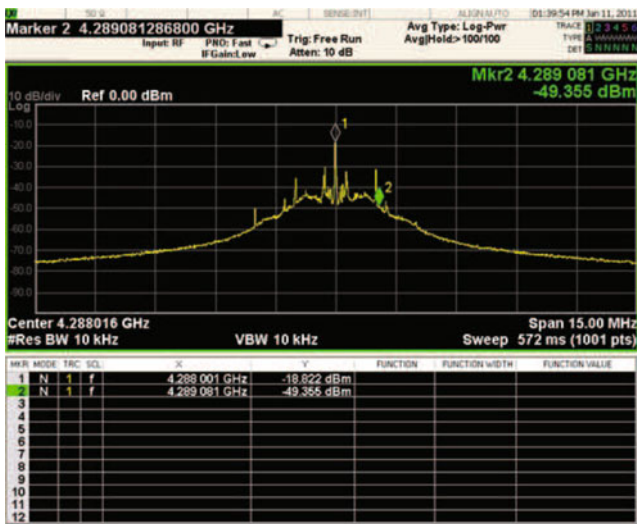
Fig. 29 PSD of PLL output with 67 MHz clock input
