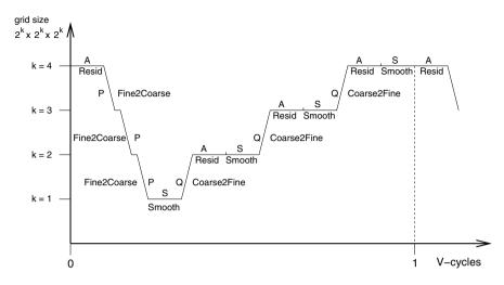
Fig. 2 Algorithmic v-cycle structure of NAS benchmark MG as a representative of multi-scale methods, reproduced from [15]
