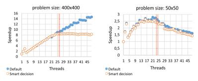
Fig. 8 Performance on AMD 48-core system with and without the proposed smart decision tool for two different problem sizes and spinning barrier implementation; smart decision tool recommendations: 26 and 24
