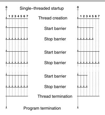
Fig. 6 Multithreaded execution: start/stop barrier model with fixed number of threads (left) and proposed model with fixed thread pool but tailor-made activations on a per with-loop basis (right)
