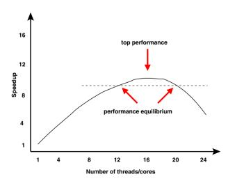
Fig. 1 Typical speedup graph observed for multi-core execution
