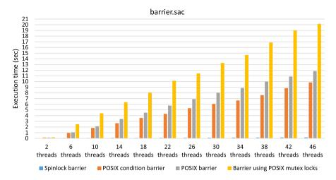
Fig. 7 Scalability of our four barrier implementations on the 48-core AMD system; our results for the Intel system are nearly identical
