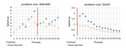
**Fig. 11** Performance on Intel 8-core hyperthreaded system with and without the proposed smart decision tool for two different problem sizes and suspending barrier implementation; smart decision tool recommendations: 9 and 1
