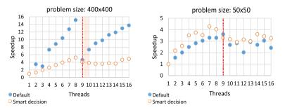
**Fig. 9** Performance on Intel 8-core hyperthreaded system with and without the proposed smart decision tool for two different problem sizes and spinning barrier implementation; smart decision tool recommendations: 9 and 9
