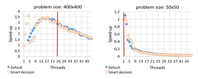
Fig. 10 Performance on AMD 48-core system with and without the proposed smart decision tool for two different problem sizes and suspending barrier implementation; smart decision tool recommendations: 24 and 1
