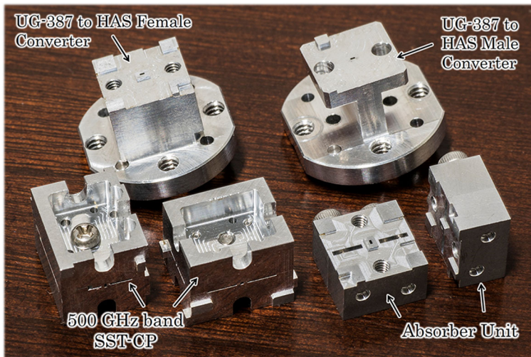
Fig. 7 Photograph of the manufactured 500-GHz SST-CP, waveguide absorber, and an HAS female to UG-387 flange converter
