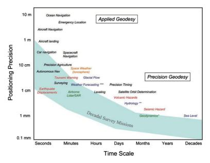
**Fig. 6** This schematic plots the precision of current applications that use spatial positioning as a function of the required time interval. The most demanding applications at the shortest time intervals include GPS seismology and tsunami warning systems. At the longest time intervals, the most demanding applications include sea level change and geodynamics [61]. (Best in color)
