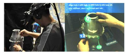
**Fig. 5** Experimental Augmented Reality Assistance for an Aircraft Engine Assembly Task. Head tracked optical see-through head-worn display overlays graphics on the user's view of components to be assembled. View through the head worn display shows dynamic 3D arors and labels that provide assistance in spatially aligning components [48]. (Best in color)
